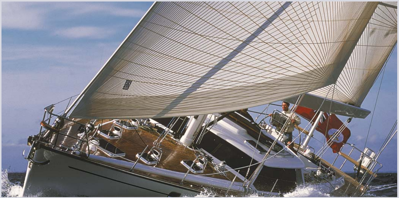
Above: A Farr Pilot House 63 with Spectra Tape-Drive sails and aramid fiber tapes. Left: The close-up shot clearly shows the Rip-Stop grid created by Tape-Drive; this sail is carbon tapes on the smoke-colored laminate. Bottom: A Seawind 1000 with Tape-Drive fathead main.
