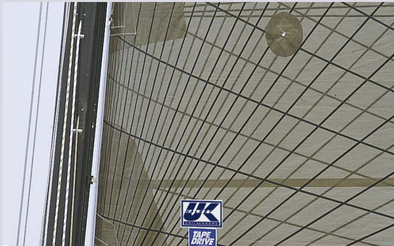
Above: A Farr Pilot House 63 with Spectra Tape-Drive sails and aramid fiber tapes. Left: The close-up shot clearly shows the Rip-Stop grid created by Tape-Drive; this sail is carbon tapes on the smoke-colored laminate. Bottom: A Seawind 1000 with Tape-Drive fathead main.
