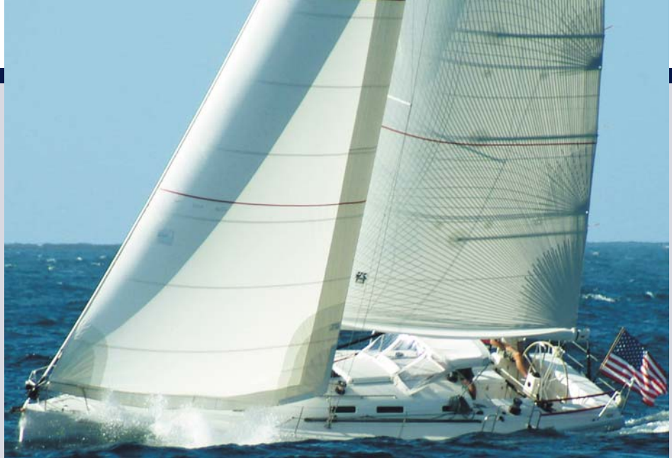
Above: J/133 with a Spectra Tape-Drive main. Below: The Oyster 68 Paper Moon crossing the Atlantic: sails are Spectra with carbon tapes.
