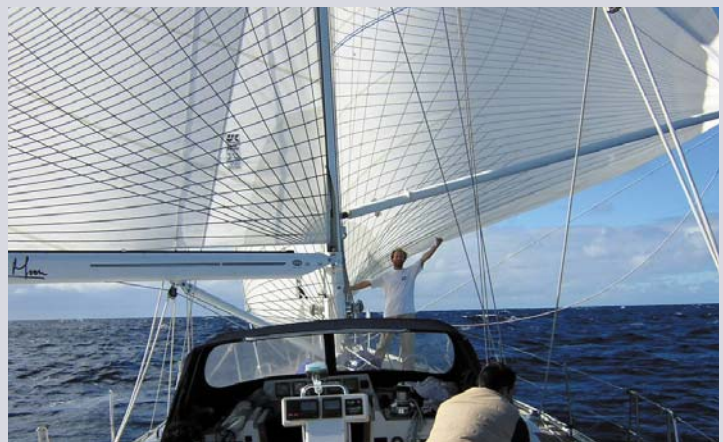
Above: J/133 with a Spectra Tape-Drive main. Below: The Oyster 68 Paper Moon crossing the Atlantic: sails are Spectra with carbon tapes.
