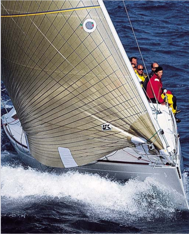
Above: Kevlar laminate with Carbon tapes. Right: One-Design class sail with Pentex laminate and Pentex tapes.
