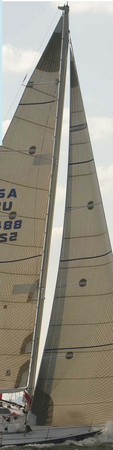
Two J/133 mains. ABOVE: Tape-Drive Titanium shape-shot. BELOW: A Tape-Drive main with carbon fiber tapes on an aramid laminate.
